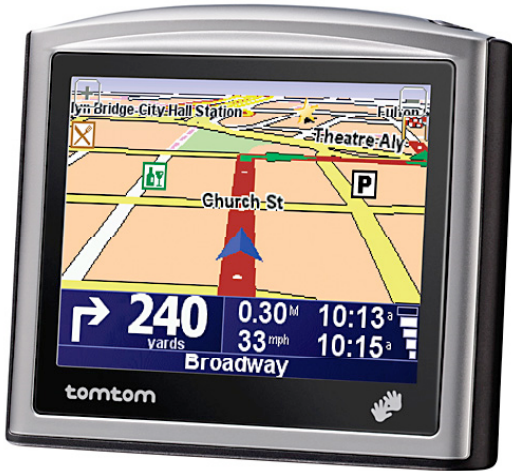
Figure 1: GPS interface displaying the next turn and the distance also its representation on the map. The other information provided on the screen are a) current speed, b) distance from destination, c) time to reach the destination and d) time of the beginning of journey.
